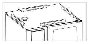
Secure the unit against slipping. The enclosed mounting kit may be used to do this.
