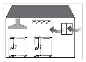
Room air-dependent gas furnaces with fans in front of burners without flow guards and total rated load in installation space less than or equal to 14kW. It is not mandatory that gas only be supplied to the burners when the exhaust system is in operation.
