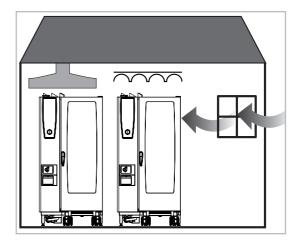
Room air-dependent gas furnaces with fans in front of burners without flow guards and total rated load in installation space greater than 14kW.
