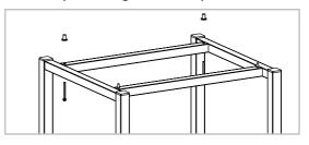
> Place the unit onto the stand. Lock the feet of the unit in place using the locating pins on the stand.
