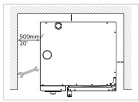
Minimum distance to other devices Minimum 350 mm distance between left side of the device and heat sources.
