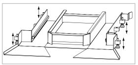
The entry ramp is attached to the right foot of the device using the ramp clamps.
