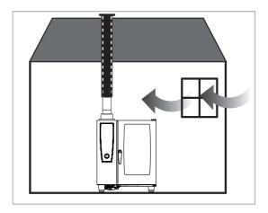
Fixed connection to a chimney is permitted if a flow guard is also in use.
