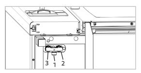
1 = 3/4" common water supply line. (cold water up to 30°C [86°F])
