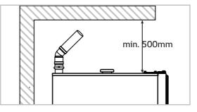
This clearance space is sufficient to install a condensation breaker so that exhaust air can be directed into non-critical areas.
