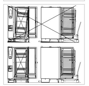
Make sure there is 200mm distance between the upper edge of the entry ramp and the floor with the unit feet.
