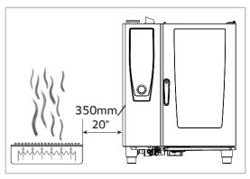
If it is not possible to keep the left side (or right, on 61 and 11) of the device a sufficient distance away from heat sources, a heat shield can reduce thermal loads.
